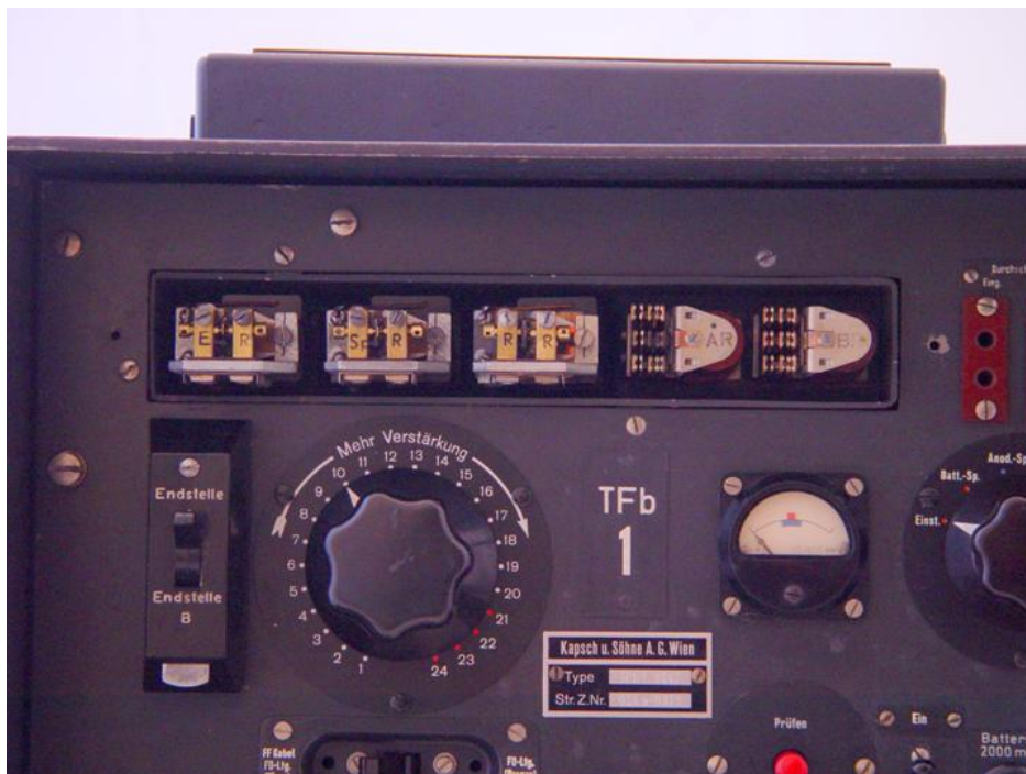
Figure 275: Ring tone generators (left) and relays (right) with relay cover
