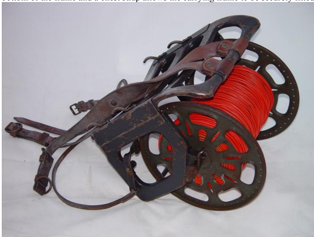
Figure 233: Collapsible model Rückentrage complete with cable drum
