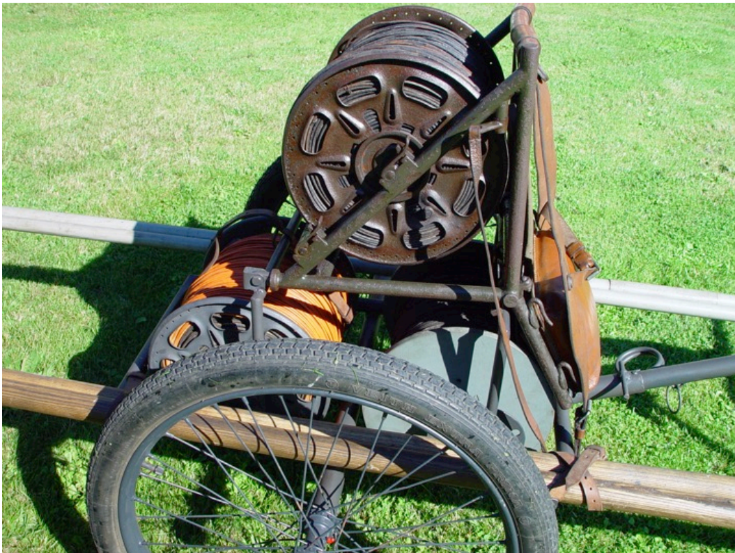
Figure 240: Cable cart with Rückentrage mounted on top. Note how pins engage the holes in the Rueckentrage
