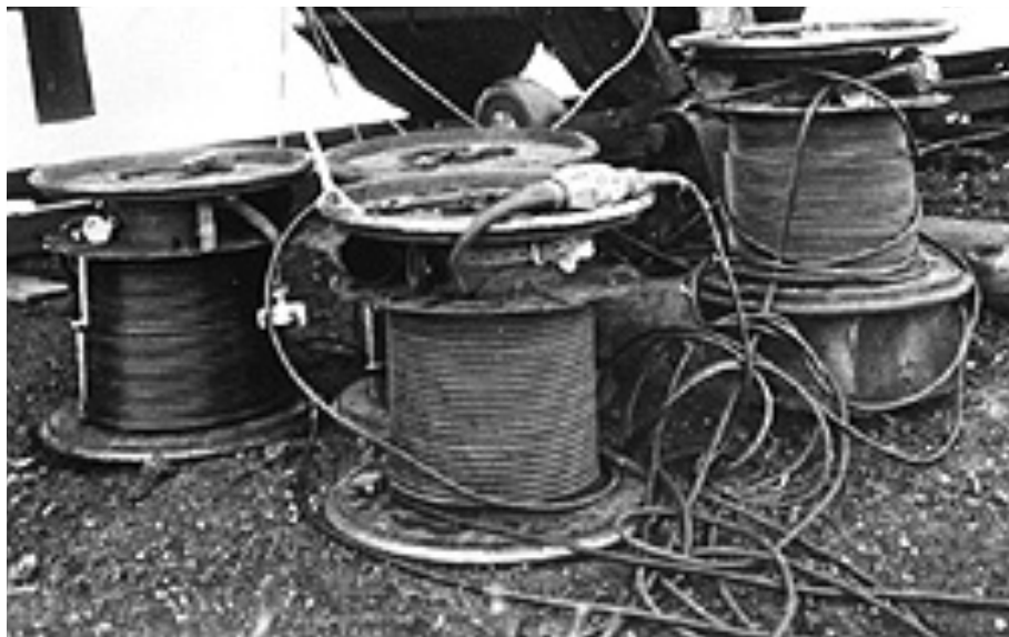
Figure 215: Several reels of Schweres Feldfernkabel at a termination point
