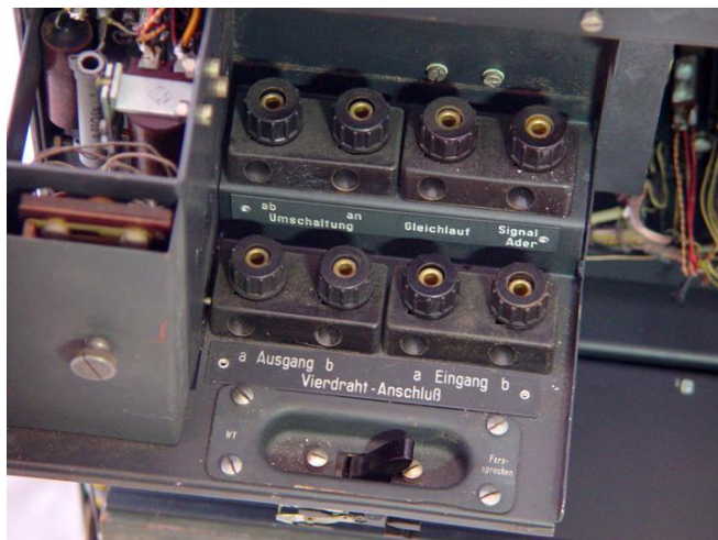
Figure 279: The Telephony - Telegraphy selection switch in the back compartment
