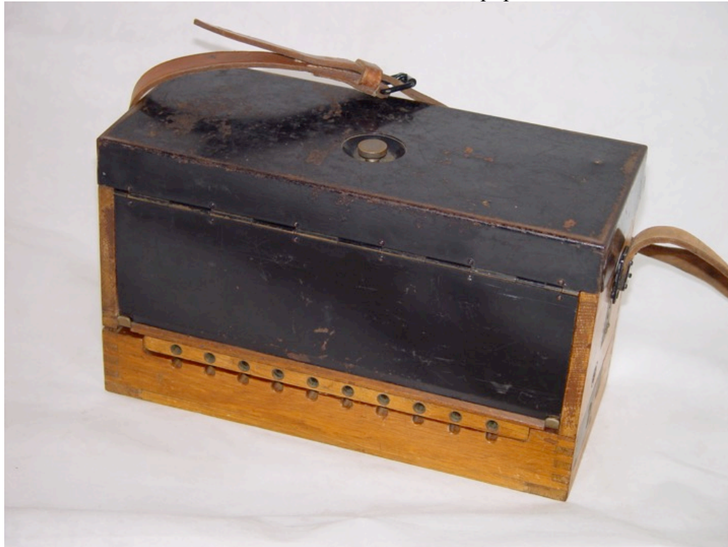
Figure 131: 10 line exchange in transport configuration
