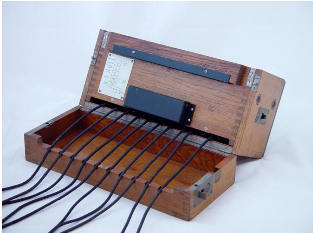
Figure 137: Klappenschrank cable storage compartment
