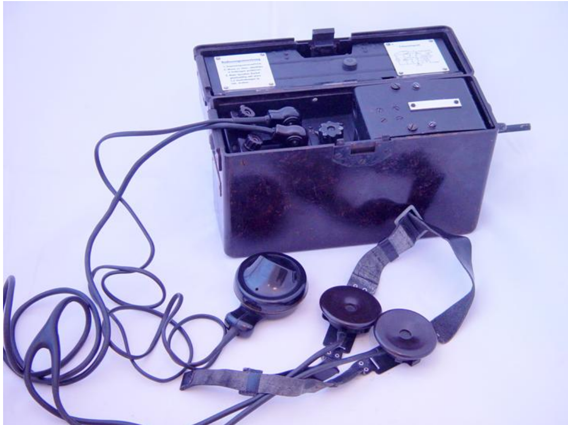
Figure 63: Erdsprechgerät with generator crank, headset and microphone connected
