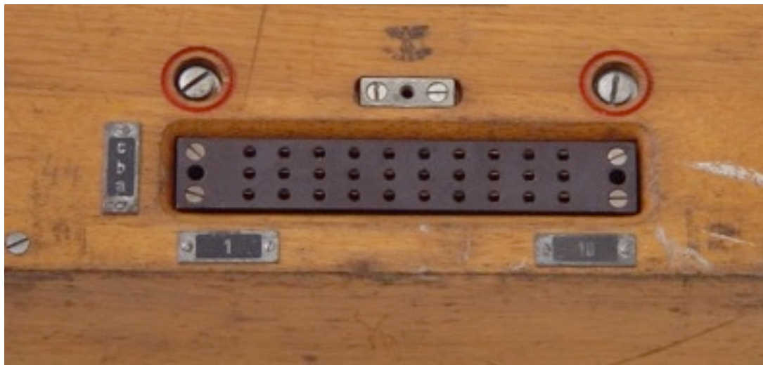
Figure 217: 30 pin socket on the back of line unit
