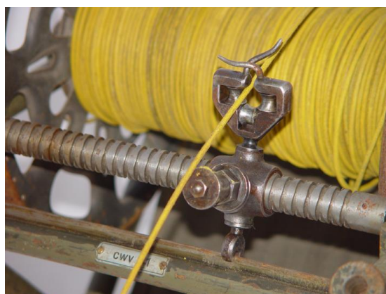
Figure 235: Cable guide on spooling axle
