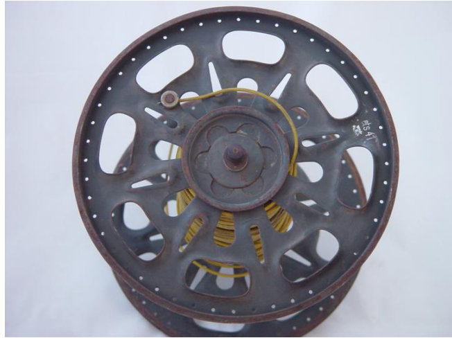
Figure 209: End of the cable connected to the drum
