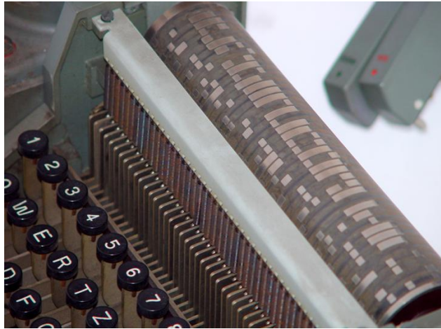
Figure 82: Keyboard and code generator
