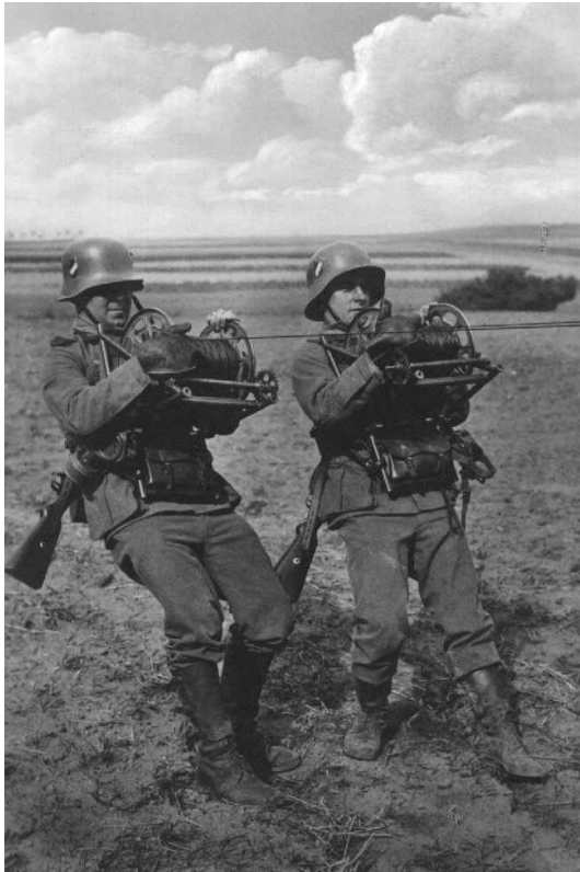
Figure 236: Rückentrage being worn on the chest. Note that the cable guide and chain are not fitted and cable gloves on the right hands
