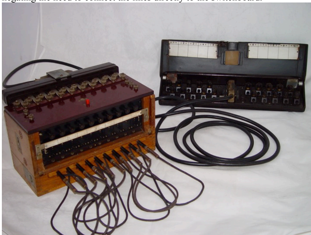
Figure 132: Remote line connection panel
