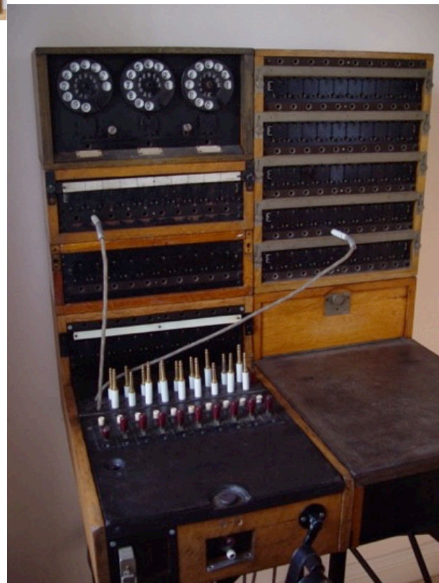
Figure 166: Configuration with 70 lines, three public connections and one conference call unit (in base unit a)
