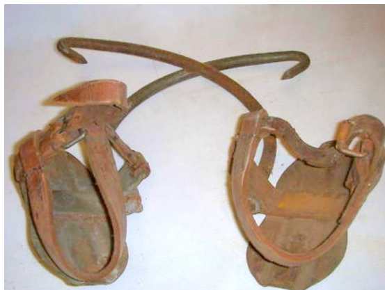
Figure 225: Climbing irons for small poles
