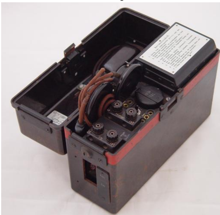
Figure 68: Sutel 40, opened lid showing the stored Morse key and headphones
