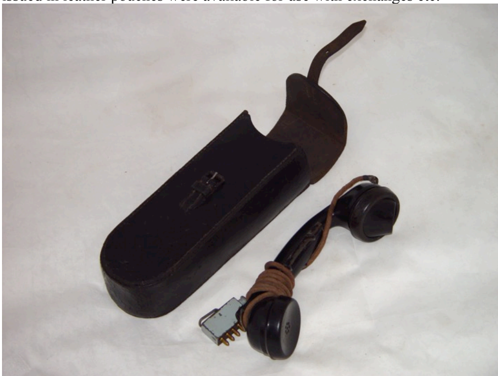
Figure 255: Handapparat 33 with leather pouch
