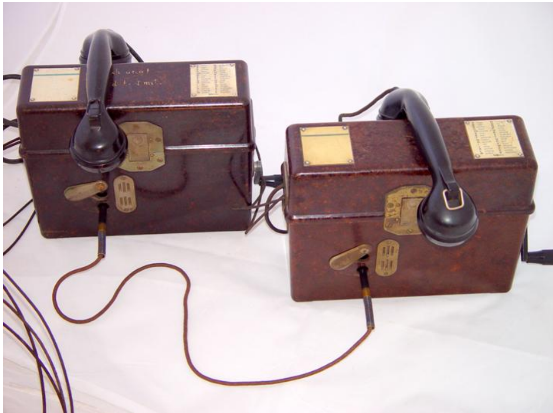
Figure 15: Two FF 33's connected by the interconnection cable
