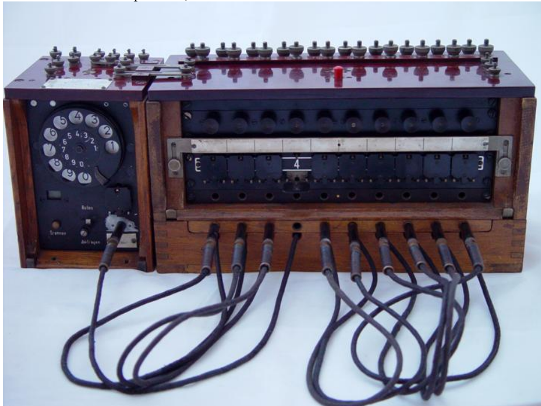
Figure 147: Line 4 of the Klappenschrank connected to an external line
