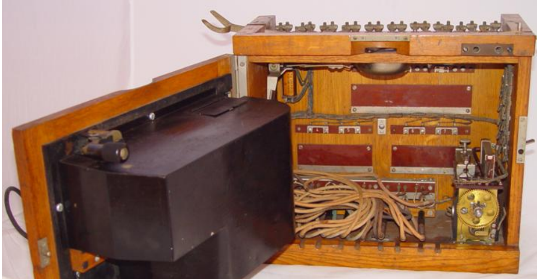
Figure 125: OB 17 front panel opened up to reveal the interior
