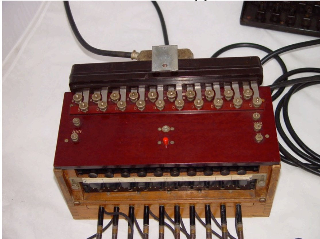
Figure 154: Laer model remote cable adaptor fitted to the 10 line exchange
