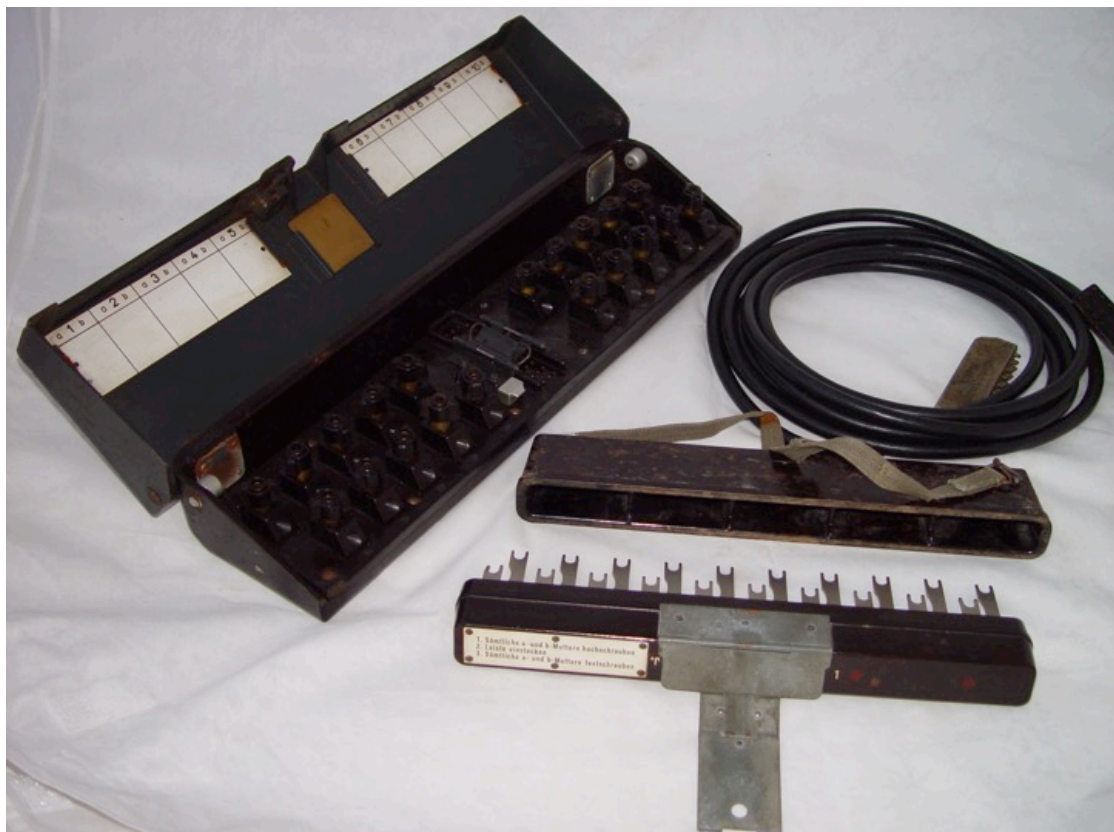
Figure 155: Later type connector, remote connection board and 30 core cable
