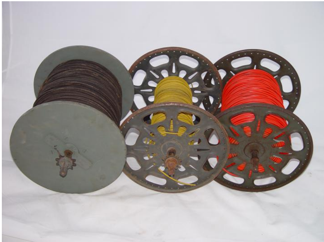
Figure 208: Various drums of heavy field cable.
