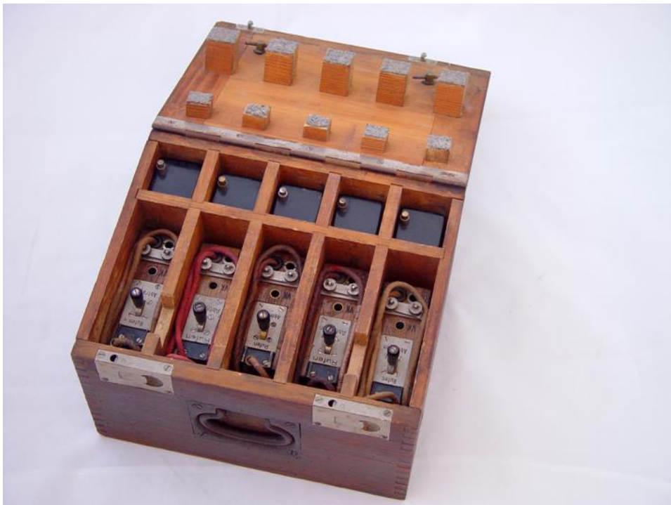
Figure 105: Five Vermittlungskästchen in box forming a five line exchange
