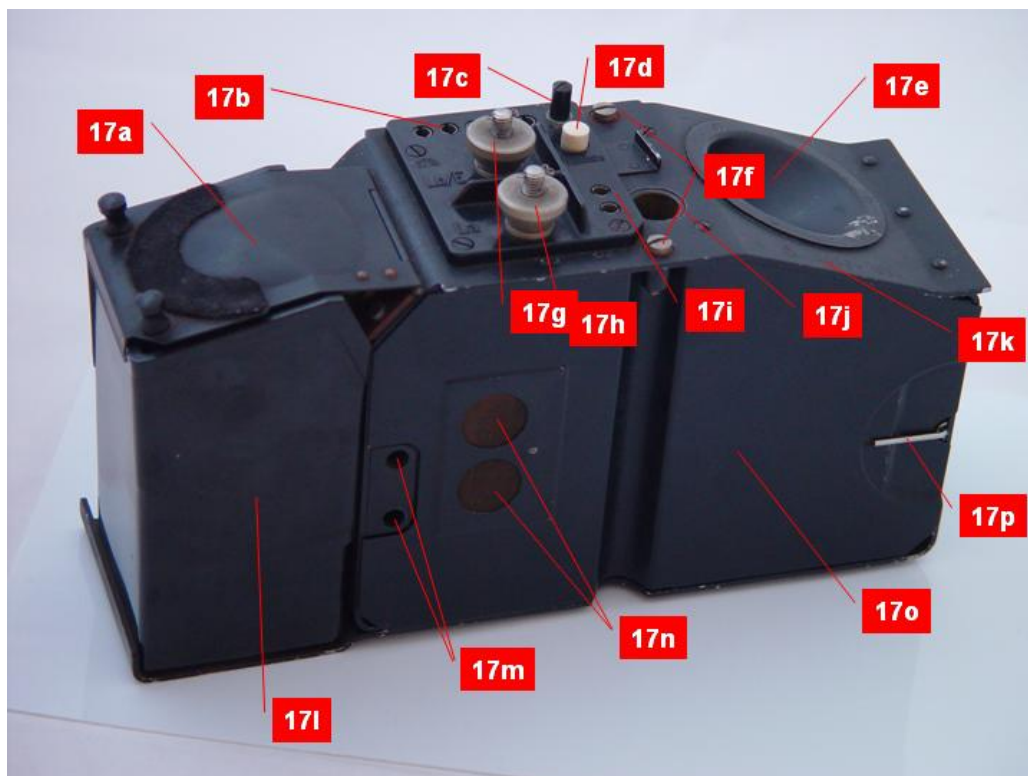
Figure 17: FF 33 telephone unit
