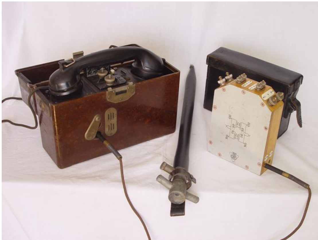
Figure 266: Übertrager connected directly to a FF 33 field telephone
