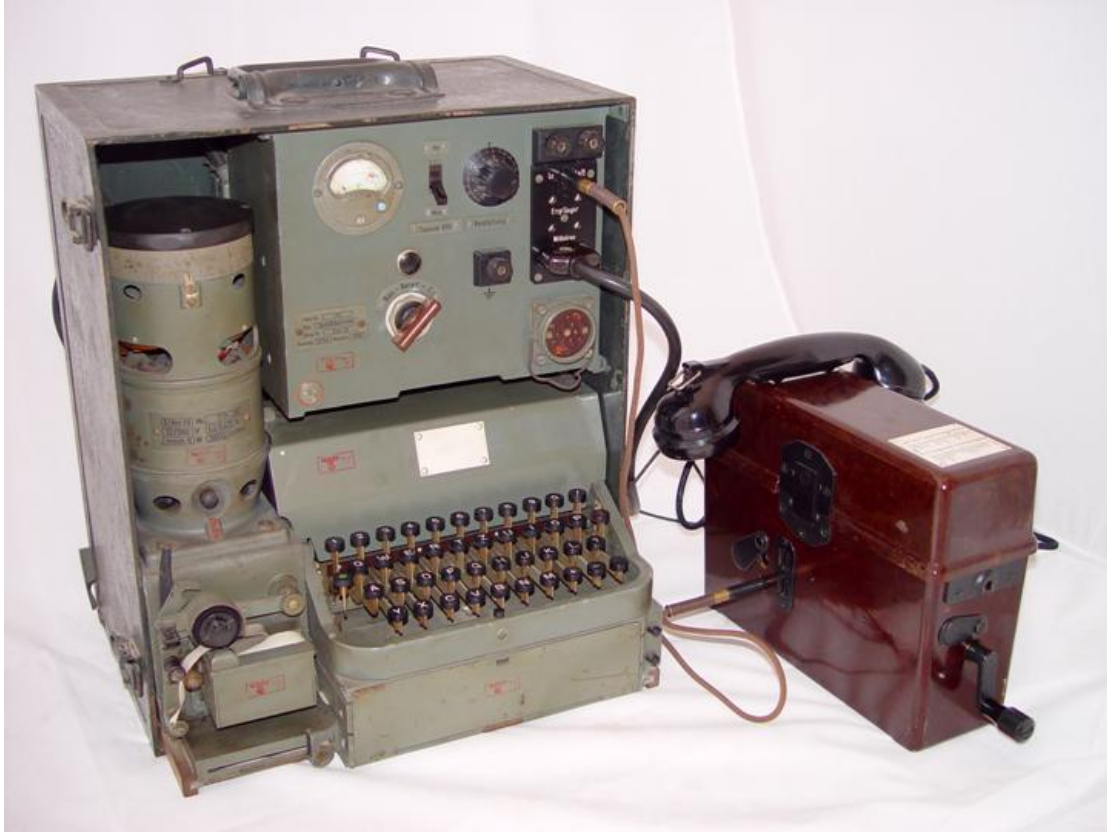
Figure 98: Feldfernschreiber plugged into an existing field telephone line
