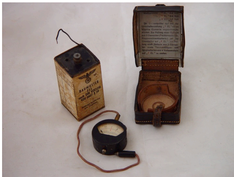
Figure 249: Elementprüfer testing a Feldelement
