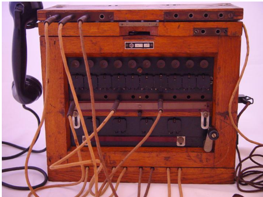
Figure 129: Lines 1, 4 and 7 connected to a conference call
