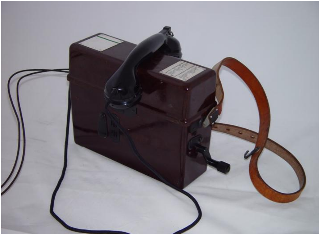
Figure 13: FF 33 connected and ready to use. Note the generator handle attached through the side and the connected carrying strap. The phone could be hung from the shoulder or a branch and the handset could be hung from the hook visible on the strap.
